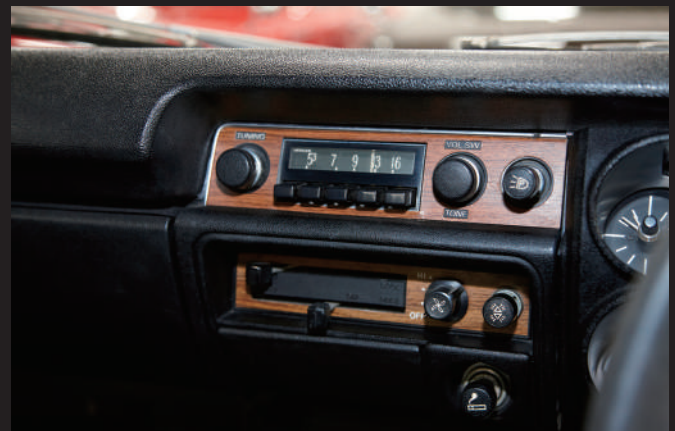
The upper section features the optional AM radio, while the lower section shows the control panel for the air conditioning, which became standard in the hardtop and includes heater functionality.
