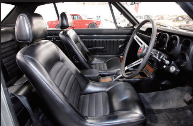
The driver and passenger seats feature fixed-back bucket seats. In the hardtop, the front seats can be tilted forward along with the seat cushion to allow access to the rear seats.
