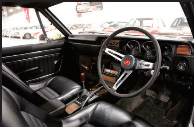
The instrument panel area shows that the hardtop has a six-gauge cluster behind the steering wheel. In the sedan version, two gauges were distributed across the center console.
